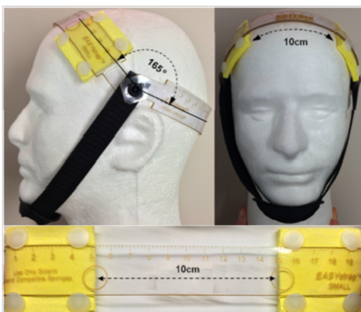
Figure 38 - OLE-system - The placement procedure is done in four steps. 1) EasyStrap size selection (small, medium, large); 2) Place the midpoint of occipital strap overinion; 3) Position the hinges that link occipital-, electrode- and chin strap over the most dorsal point on the ear; 4) Adjust the angle between occipital and electrode strap to 165 and the distance across the stars between the dorsal electrode edges to 10cm. Adapted from Seibt et al, 2015.
